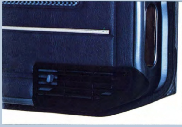
Air exit vent for flow-through ventilation.
